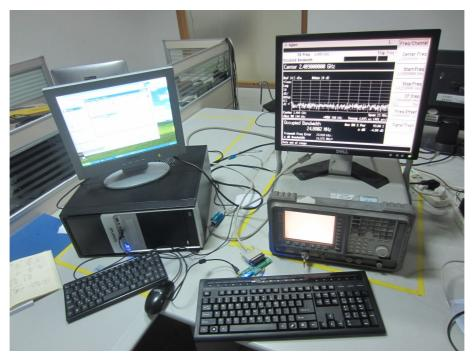
CONDUCTED EMISSION TEST SETUP
