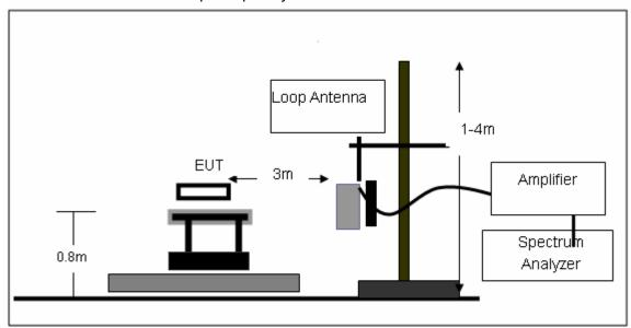
(B) Radiated Emission Test-Up Frequency 30MHz~1GHz
