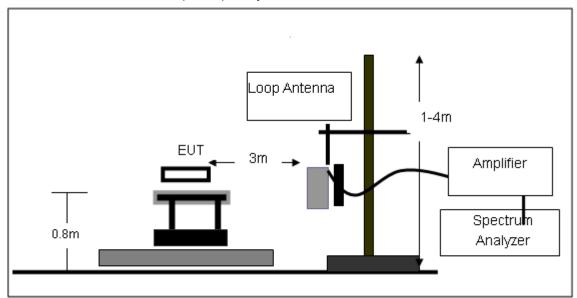
(B) Radiated Emission Test-Up Frequency 30MHz~1GHz
