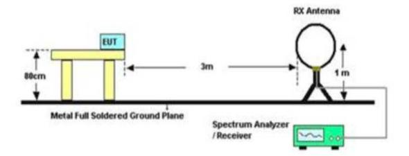
(B) Radiated Emission Test-Up Frequency 30MHz~1GHz
