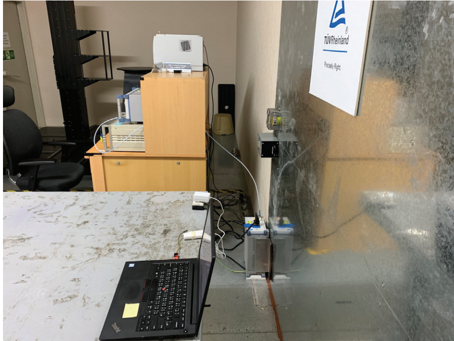
Photograph 7: Set-up for Mains Conducted testing (Back View)
