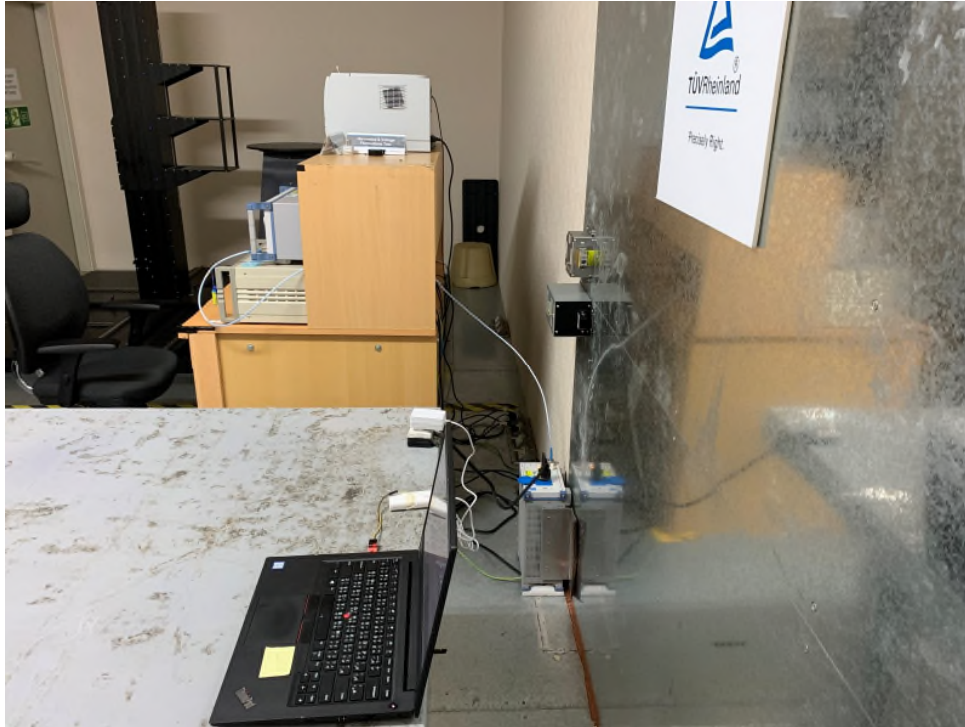
Photograph 7: Set-up for Mains Conducted testing (Back View)
