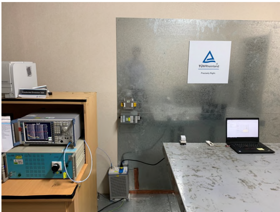
Photograph 8: Set-up for Mains Conducted testing (Front View)
