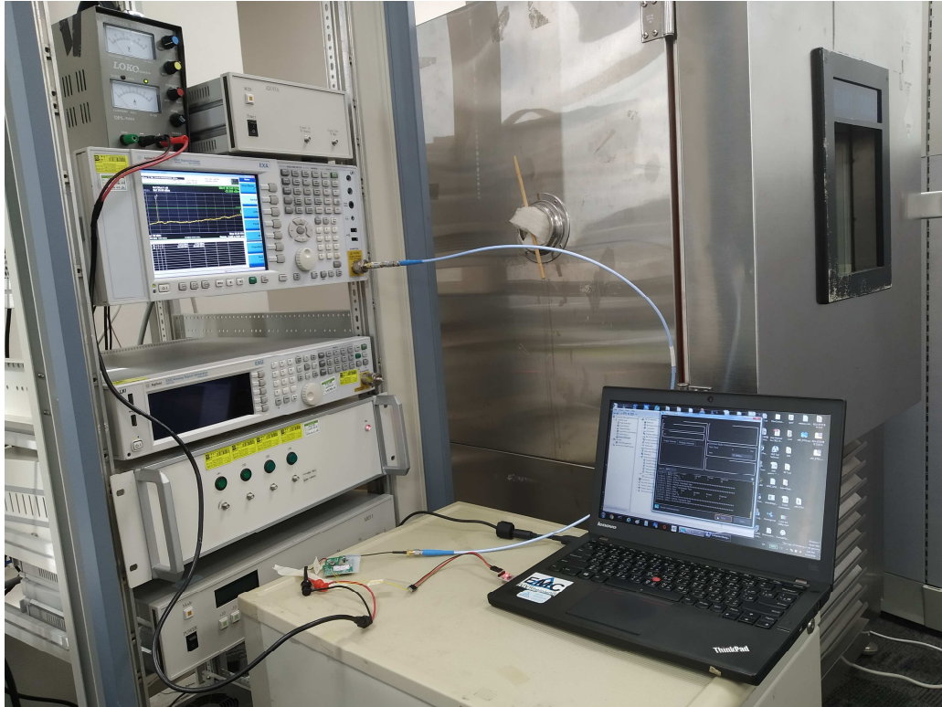
Photograph 5: Set-up for Conducted testing
