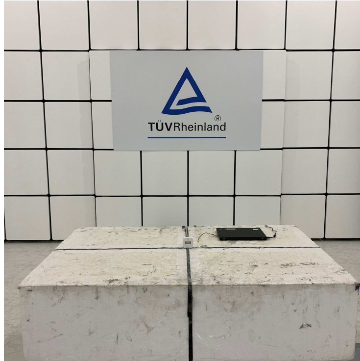
Photograph 2: Set-up for Spurious Emissions (Back View 1)
