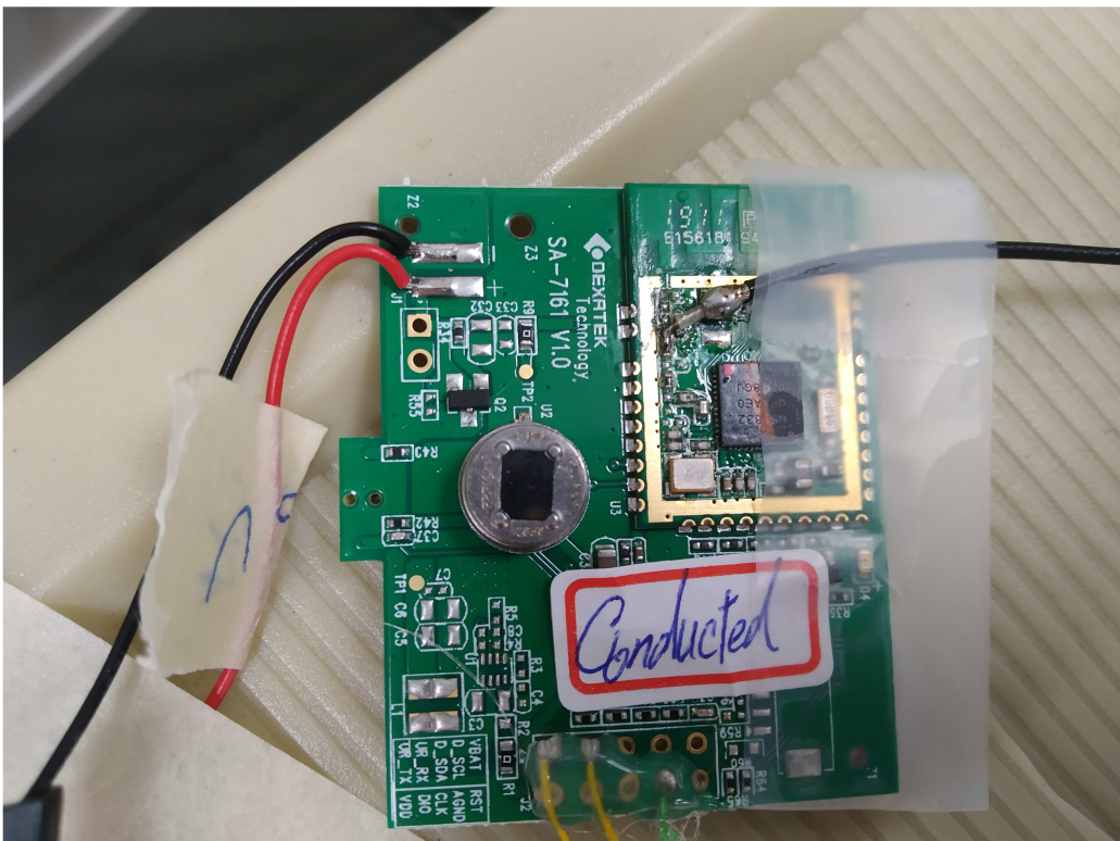
Photograph 6: Set-up for Conducted testing
