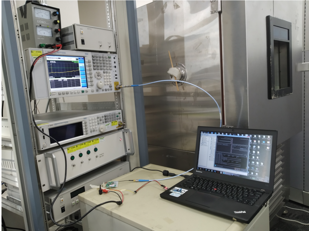
Photograph 5: Set-up for Conducted testing
