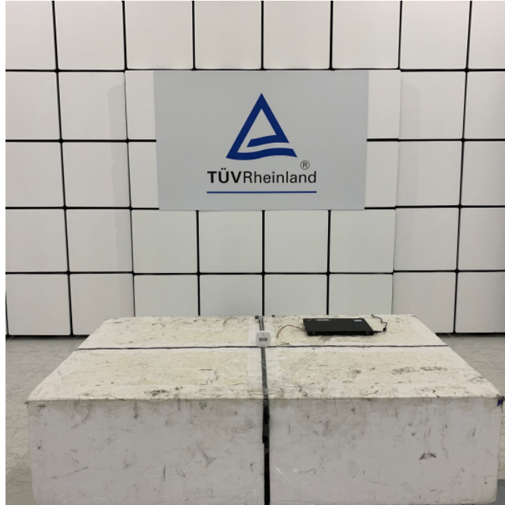
Photograph 2: Set-up for Spurious Emissions (Back View 1)
