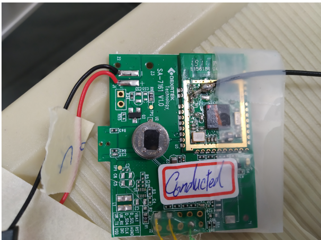
Photograph 6: Set-up for Conducted testing
