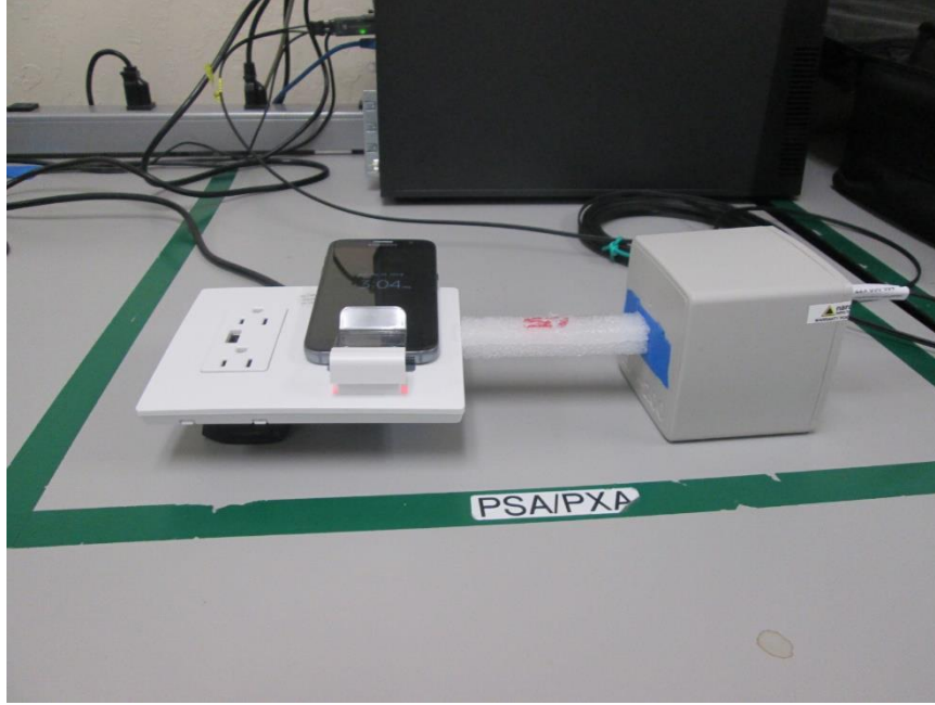
S2, RF EXPOSURE SETUP PHOTO 15cm
