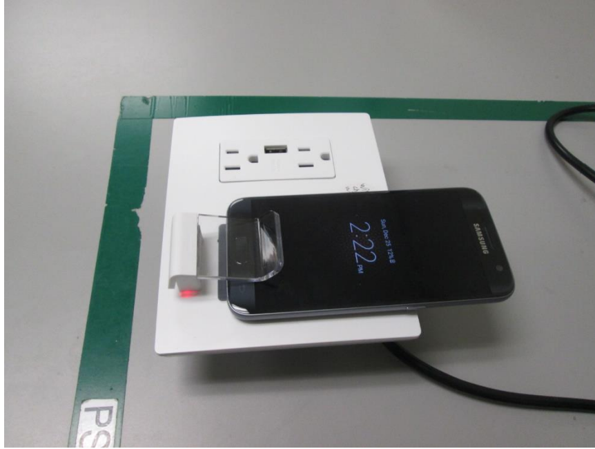
COIL1, RF EXPOSURE SETUP PHOTO
