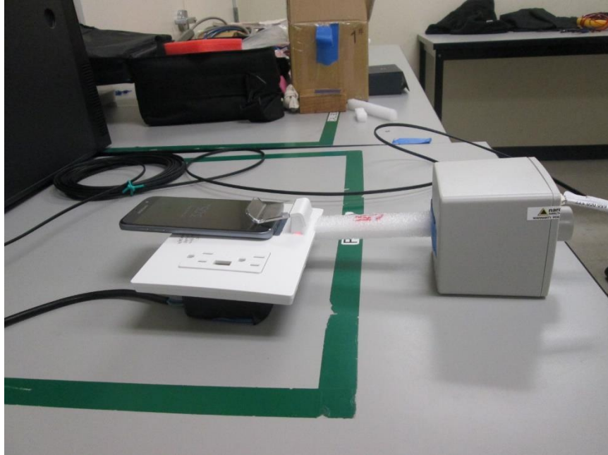
S3, RF EXPOSURE SETUP PHOTO 15cm
