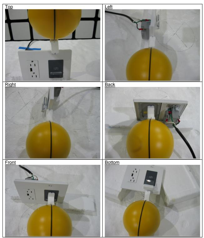
**Note**: A foam spacer was added to the tip of probe to maintain 10cm spacing between the reference point of the probe and the EUT.
