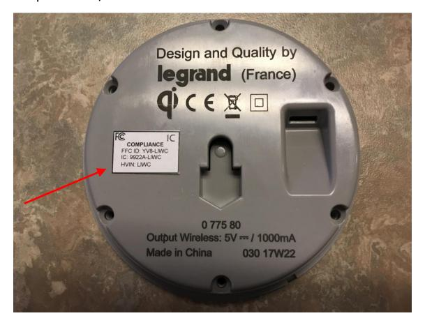
Proposed Secondary FCC/IC Label on Mounting Plate:
