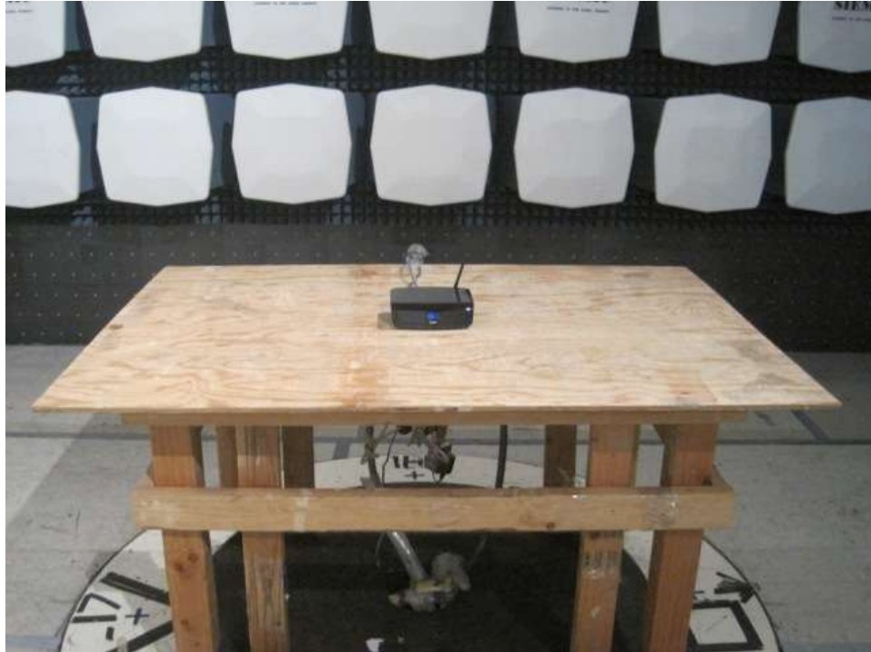
Radiated Emission (>1GHz) Setup Front View
