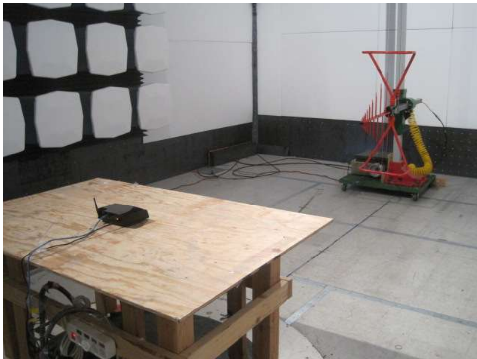
Radiated Emission Rear View (30MHz-1GHz)
