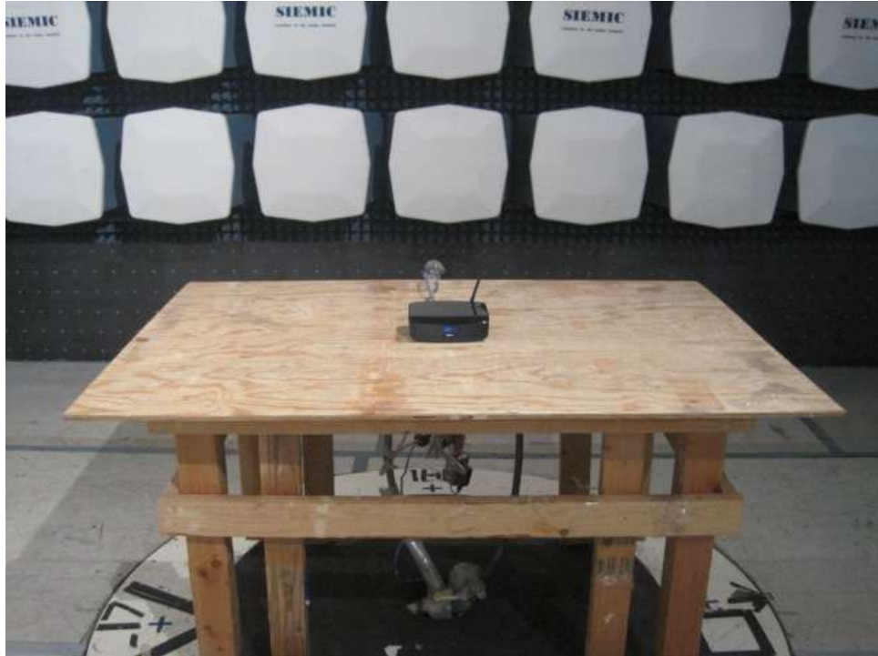
Radiated Emission Front View (30MHz-1GHz)
