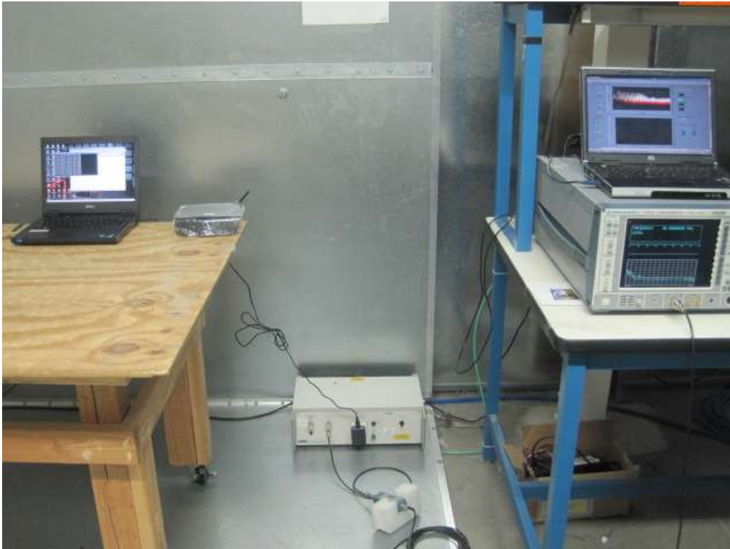
Conducted Emission Setup View
