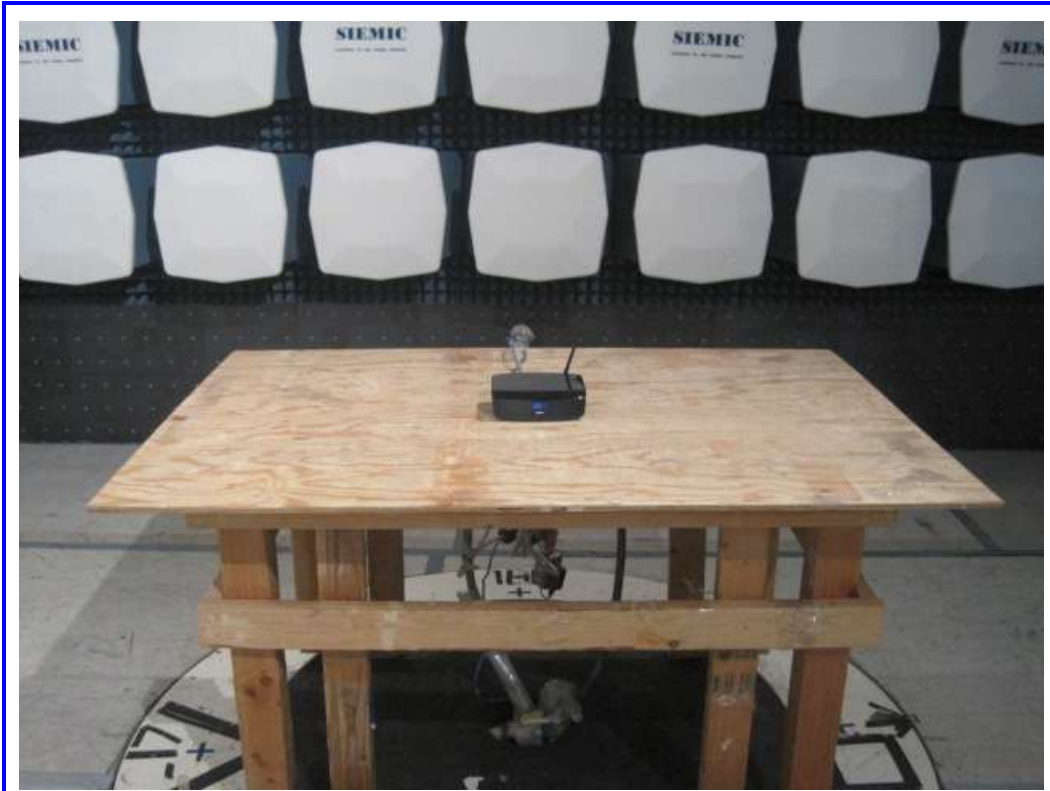
Radiated Emission (<1GHz) Setup Front View
