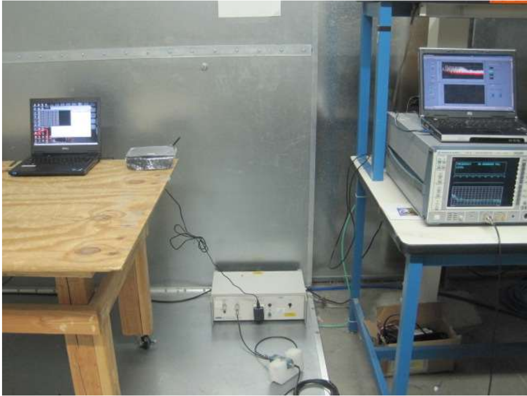
Conducted Emission Setup View
