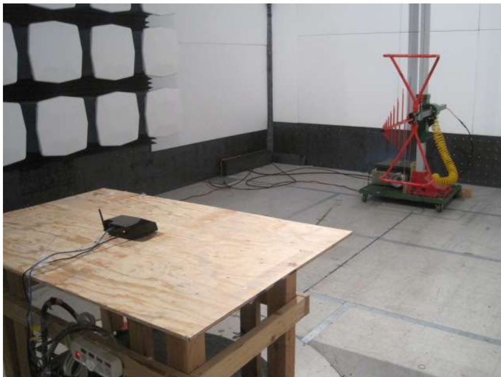
Radiated Emission (<1GHz) Setup Rear View
