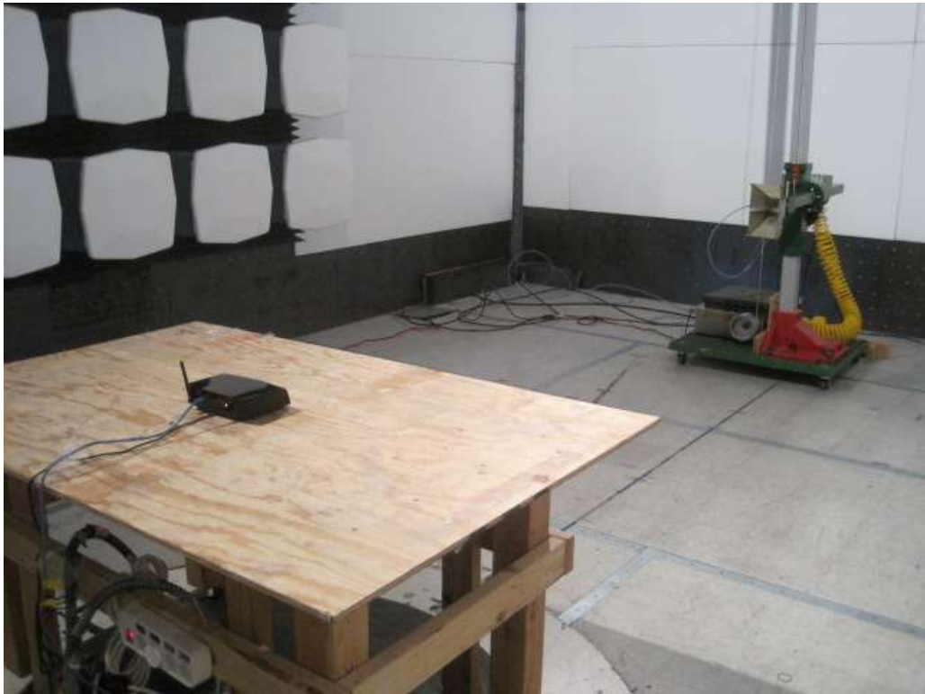
Radiated Emission (>1GHz) Setup Rear View
