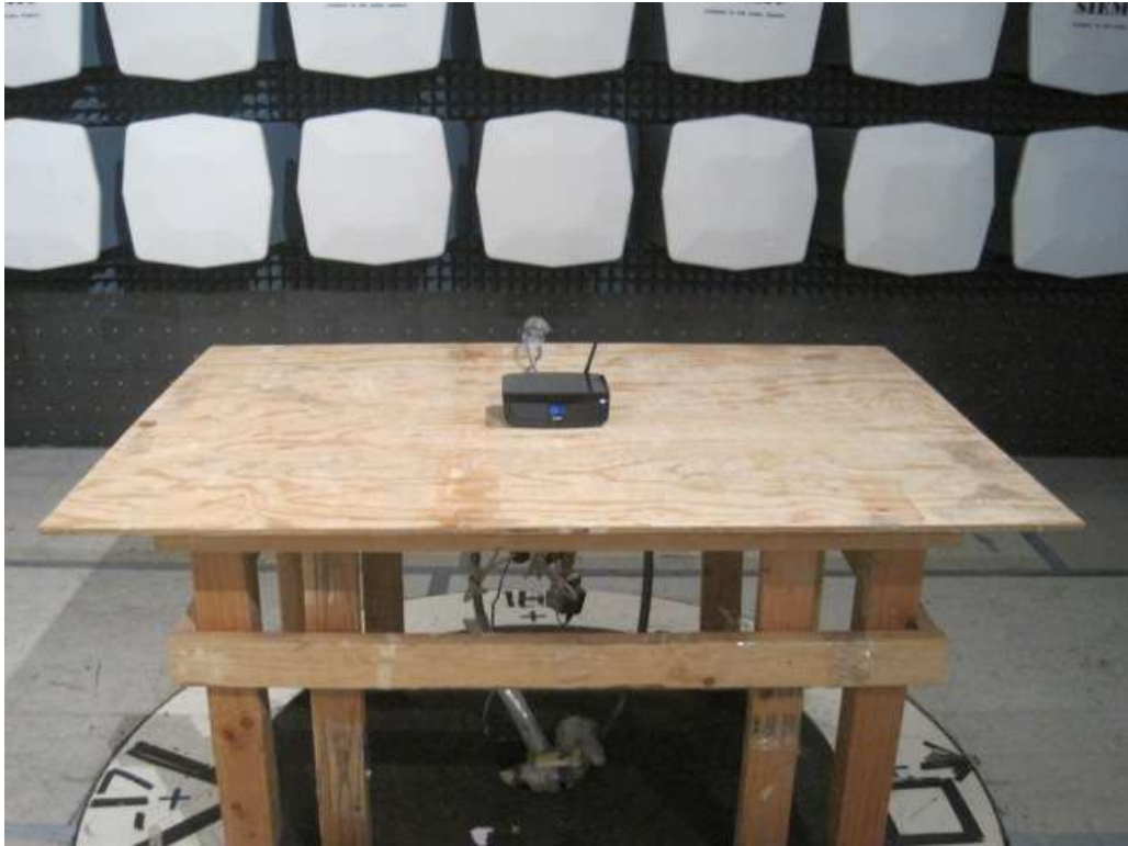
Radiated Emission (>1GHz) Setup Front View
