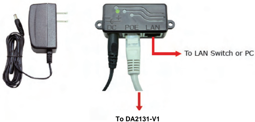
Figure 2-4 Connect to PoE Injector
