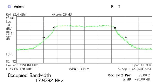
Transmit Freq Error 107.168 kHz x dB Bandwidth 22.139 MHz
