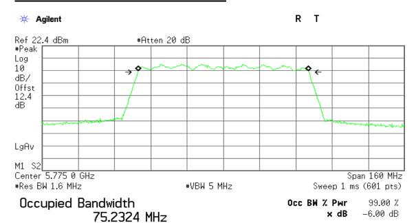
Transmit Freq Error 36.673 kHz x dB Bandwidth 75.593 MHz
