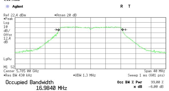
Transmit Freq Error 33.145 kHz x dB Bandwidth 16.570 MHz
