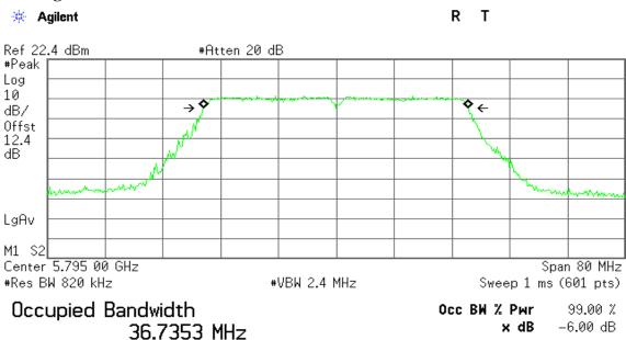
Transmit Freq Error -63.376 kHz x dB Bandwidth 36.683 MHz
