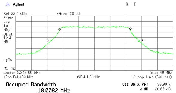
Transmit Freq Error 146.174 kHz x dB Bandwidth 22.337 MHz
