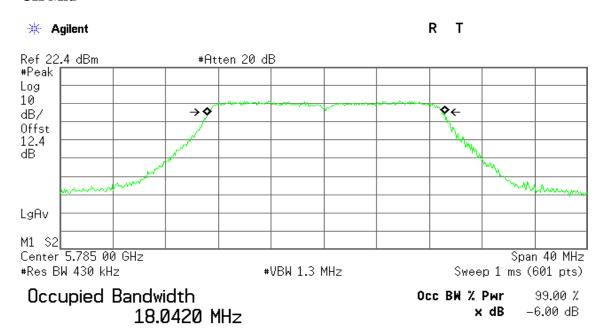
Transmit Freg Error 160.073 kHz x dB Bandwidth 17.762 MHz
