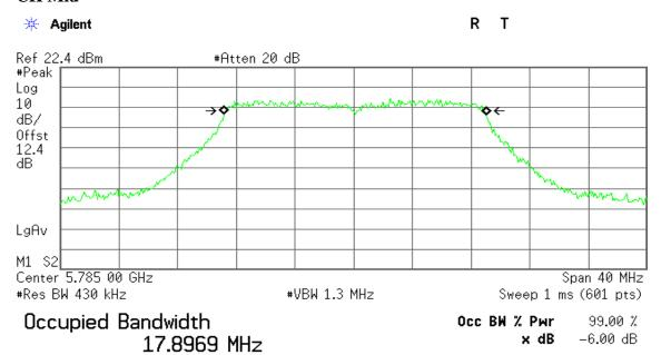
97.356 kHz Transmit Freq Error x dB Bandwidth 17.675 MHz
