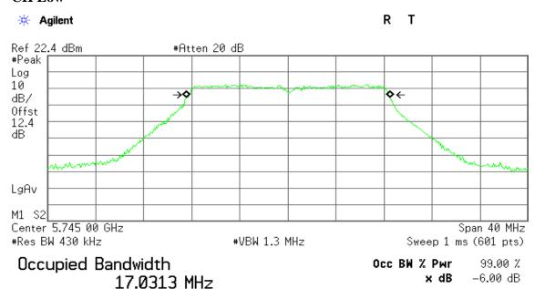
Transmit Freq Error 20.309 kHz x dB Bandwidth 16.574 MHz
