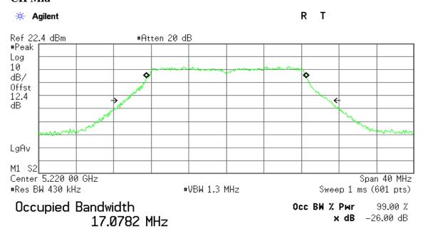
Transmit Freq Error 23.451 kHz x dB Bandwidth 21.752 MHz
