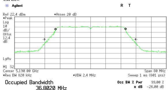
Transmit Freq Error 66.784 kHz x dB Bandwidth 44.415 MHz
