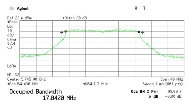
Transmit Freq Error 100.889 kHz x dB Bandwidth 17.699 MHz
