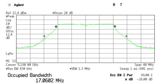
Transmit Freq Error 11.063 kHz x dB Bandwidth 21.946 MHz
