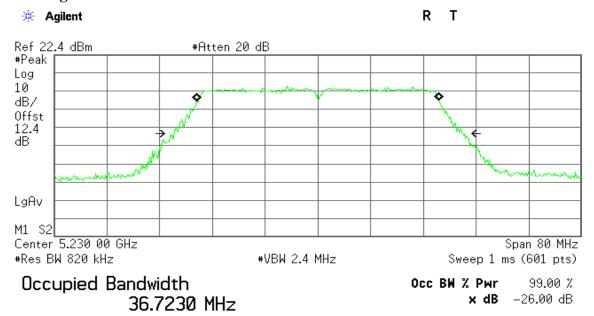
Transmit Freq Error 27.768 kHz x dB Bandwidth 43.820 MHz
