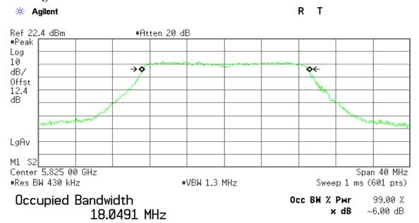
Transmit Freq Error 153.909 kHz x dB Bandwidth 17.709 MHz
