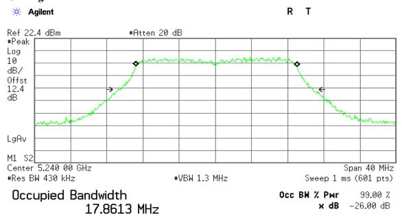
Transmit Freq Error 110.086 kHz x dB Bandwidth 21.502 MHz
