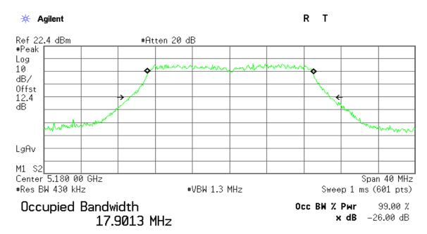
Transmit Freq Error 91.513 kHz x dB Bandwidth 21.503 MHz
