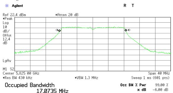
Transmit Freq Error -21.572 kHz x dB Bandwidth 16.573 MHz
