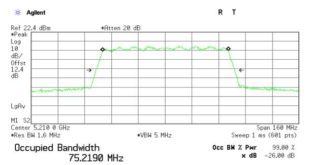
Transmit Freq Error 197.864 kHz x dB Bandwidth 82.774 MHz
