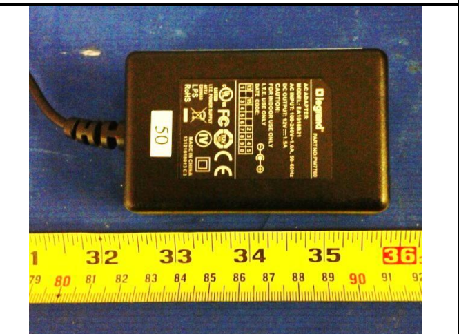
Power Supply – Bottom View
