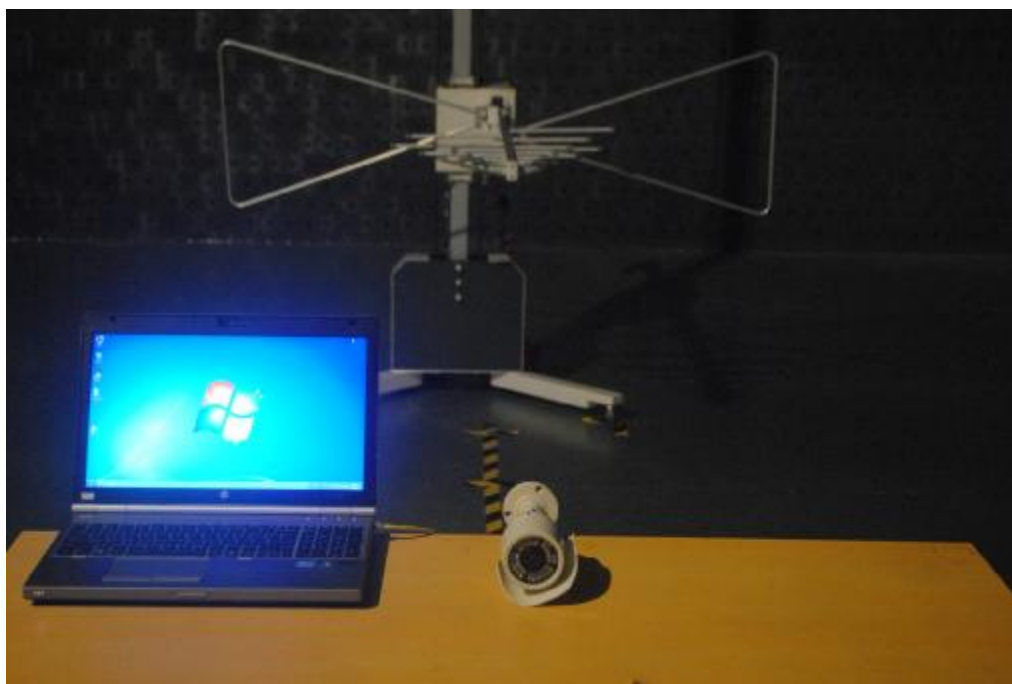
Radiated emission test view
