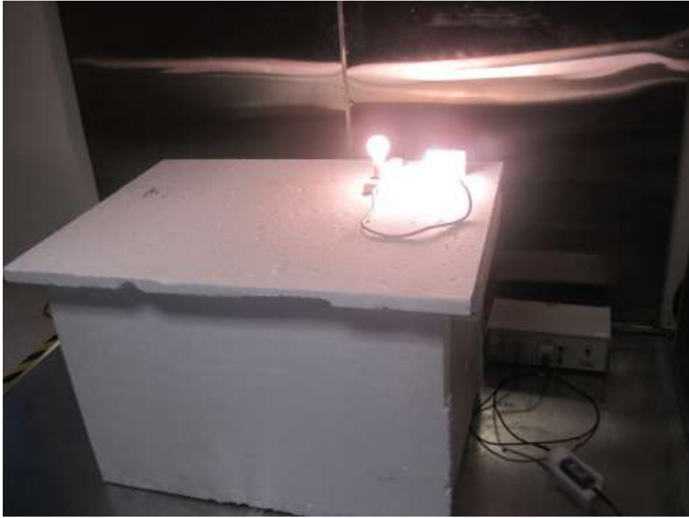
Conducted Emission Setup Front View
