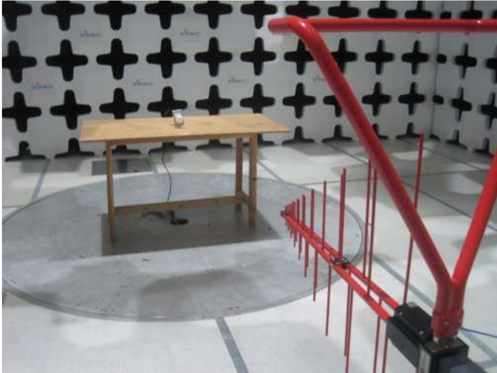
Radiated Emission Front View (30MHz-1GHz)
