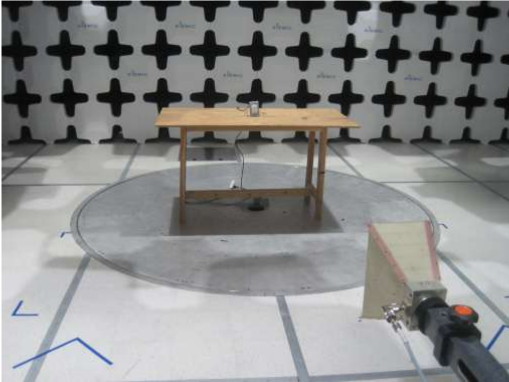
Radiated Emission (>1GHz) Setup Front View
