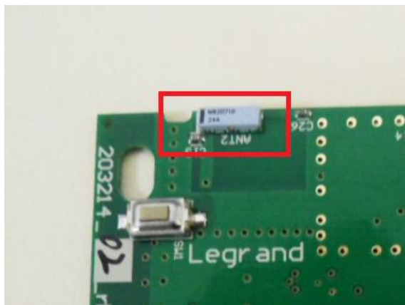
Antenna close View
