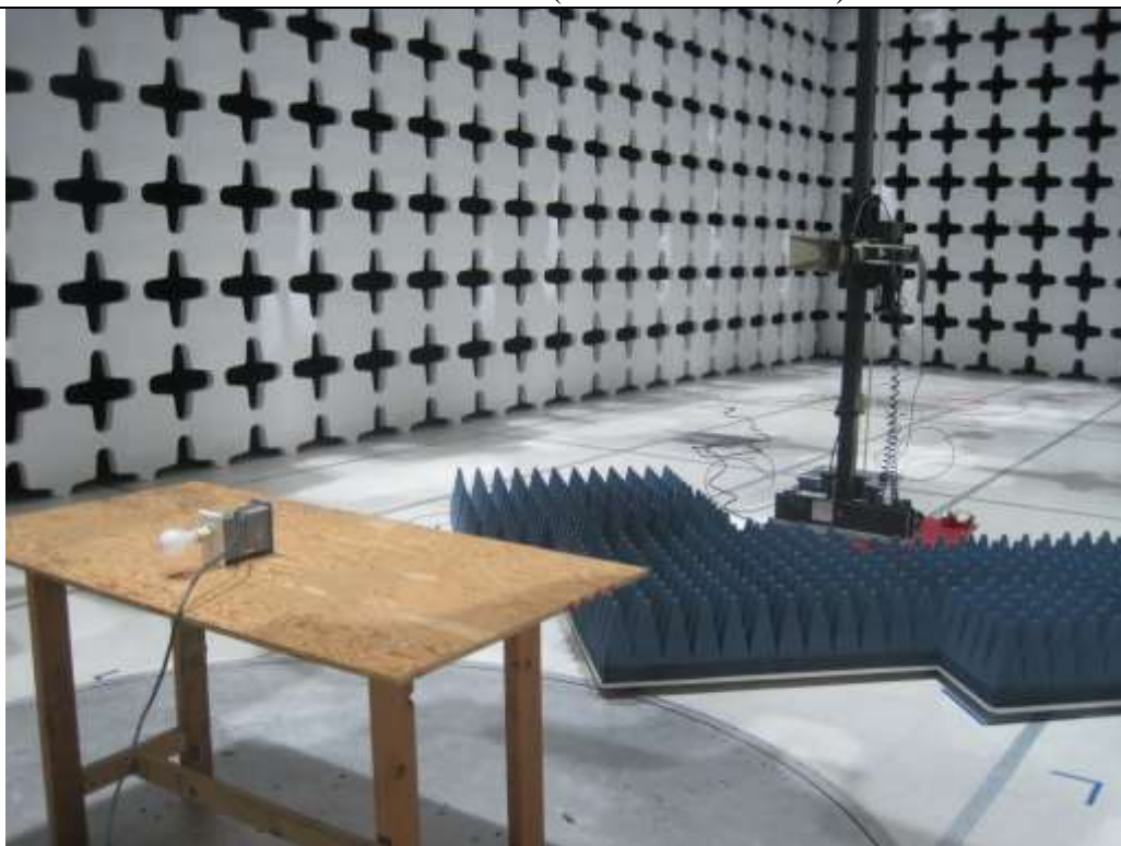
Radiated Emission above 1GHz (ADTP600RMHW1) - Rear View
