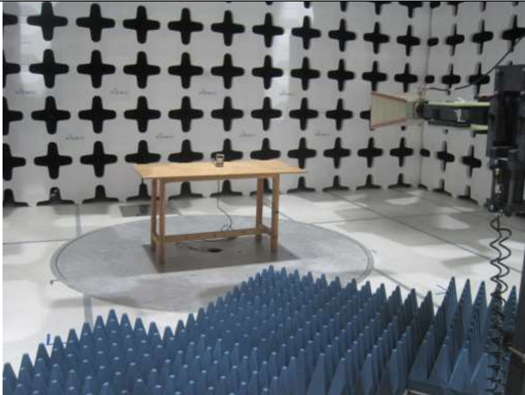
Radiated Emission above 1GHz (ADTH700RMTUW1) - Front View
