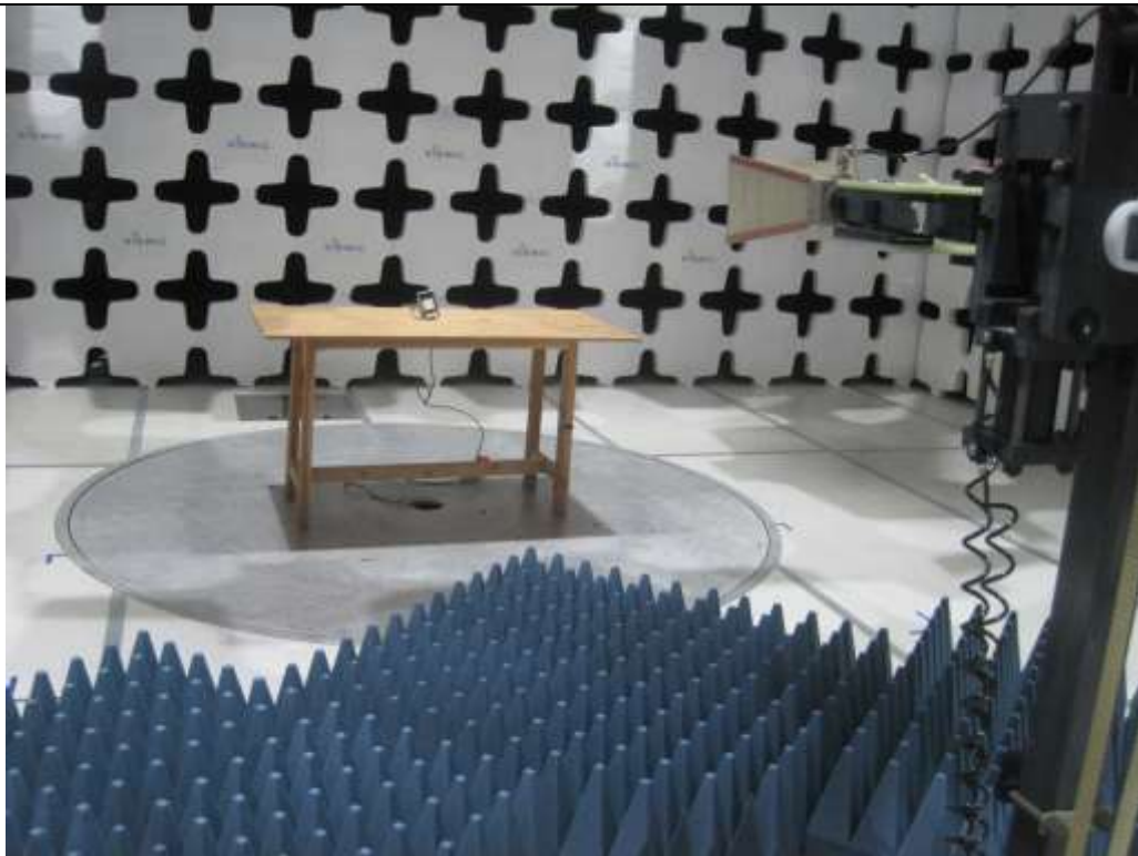
Radiated Emission above 1GHz (ADTP700RMUW1) - Front View
