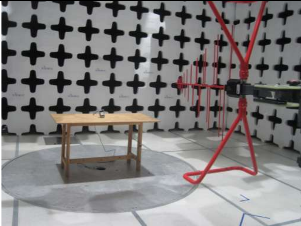
Radiated Emission below 1GHz - Front View
