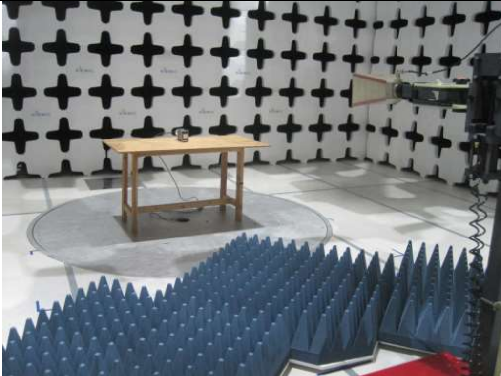
Radiated Emission above 1GHz (ADTP600RMHW1) - Front View
