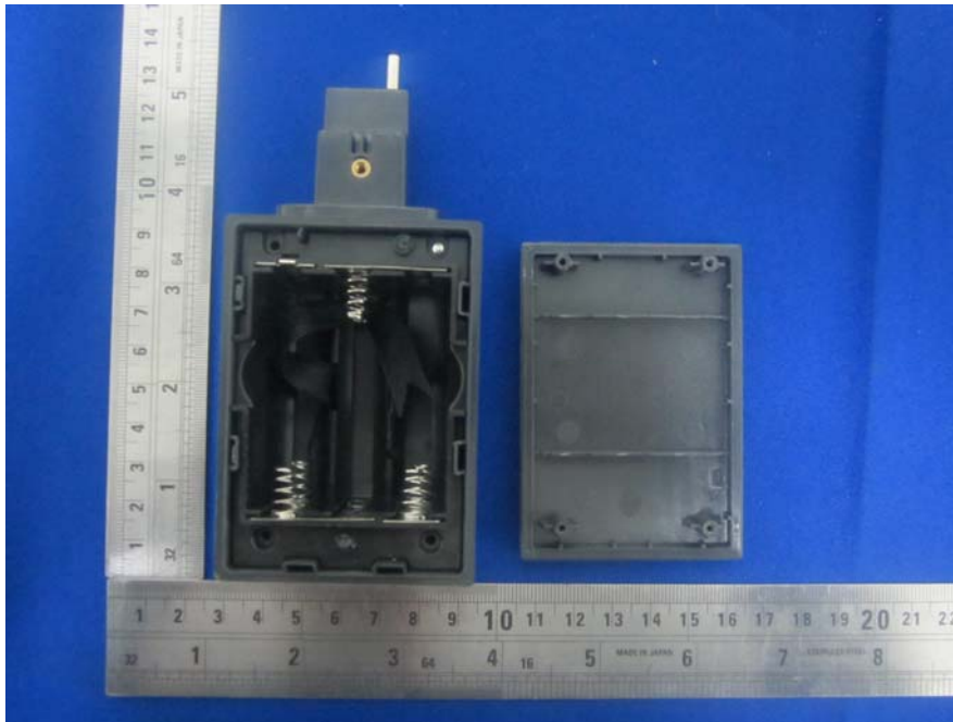
EUT –Battery Box Uncover View
