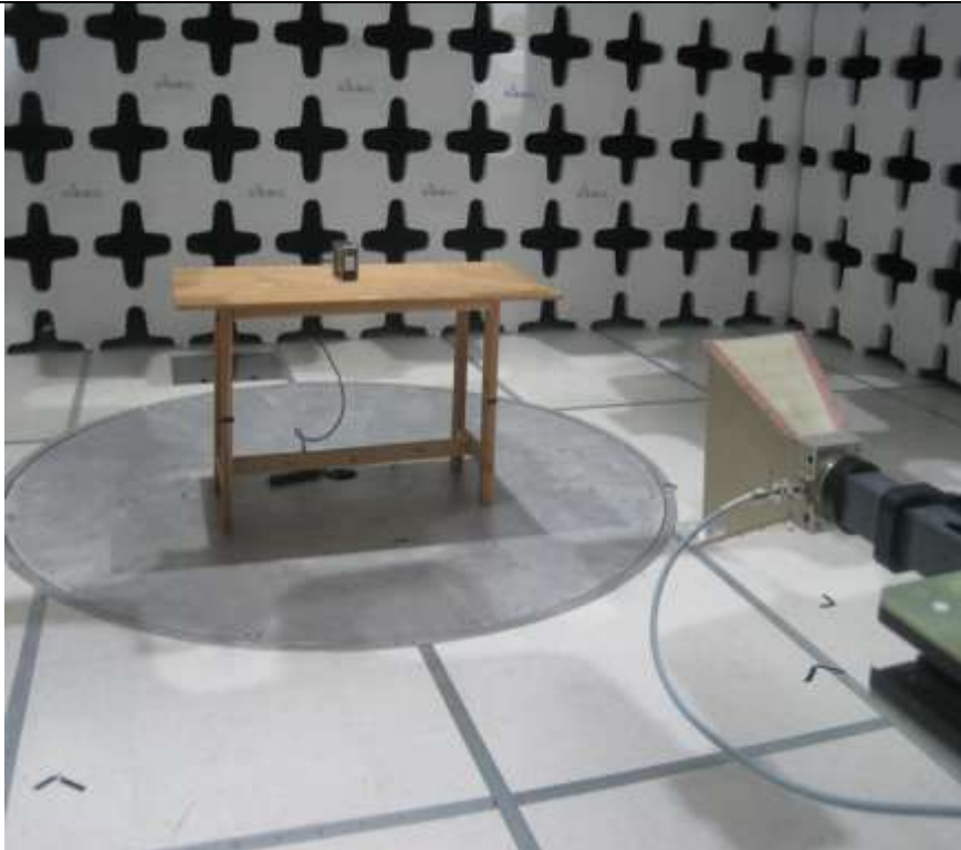
Radiated Emission above 1GHz (ADTP700MMHW2) - Front View
