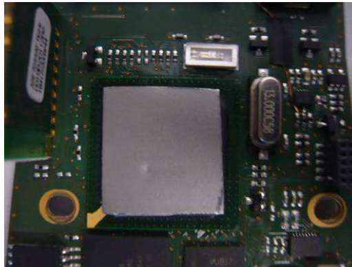
Conductive foam on chip
