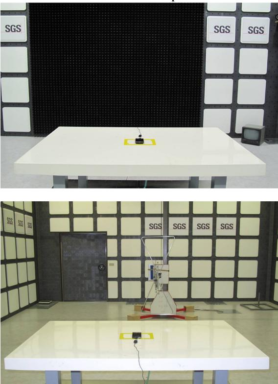
**Radiated Emission Set up Photo**
