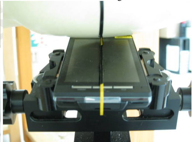
Fig.6 Left Head Section / Ear-Tilt Position(15°)
