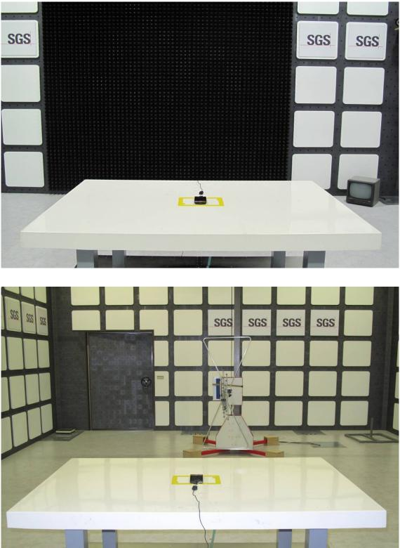
**Radiated Emission Set up Photos**
