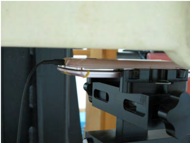
Fig.13 Body worn - EUT back to flat phantom and distance between flat phantom and mobile phone is 1.5 cm_ repeated with headset.
