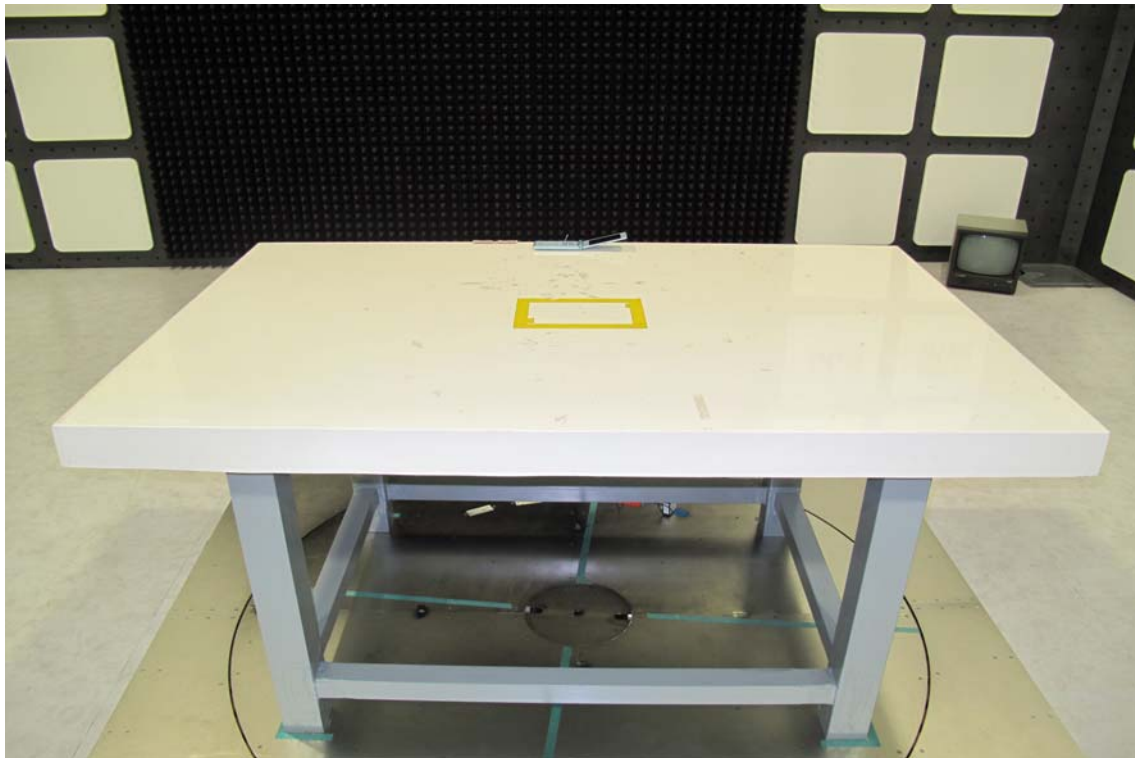
Radiated Emission Test Setup Photo (config 3)
