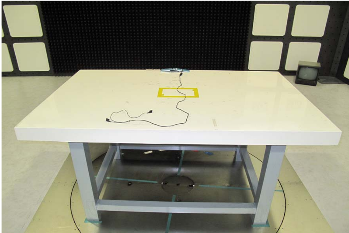
Radiated Emission Test Setup Photo (config 2)
