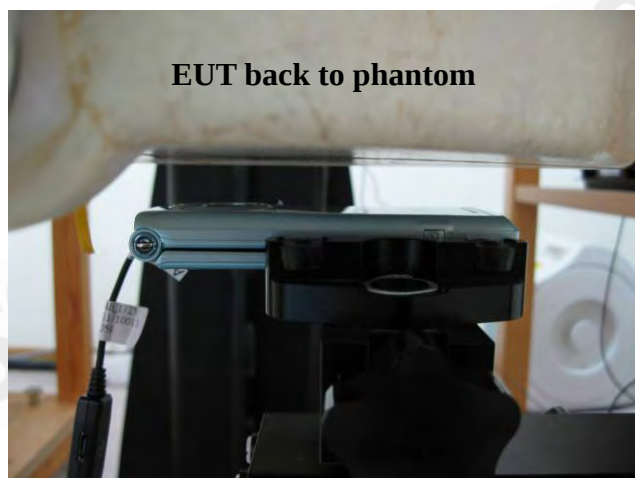
Fig.9 Body worn- EUT front to flat phantom and distance between flat phantom and mobile phone is 1.5 cm_ repeated with Headset.
