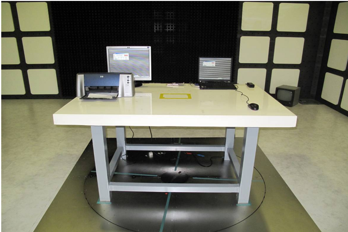
Radiated Emission Test Setup Photo (config 5)
