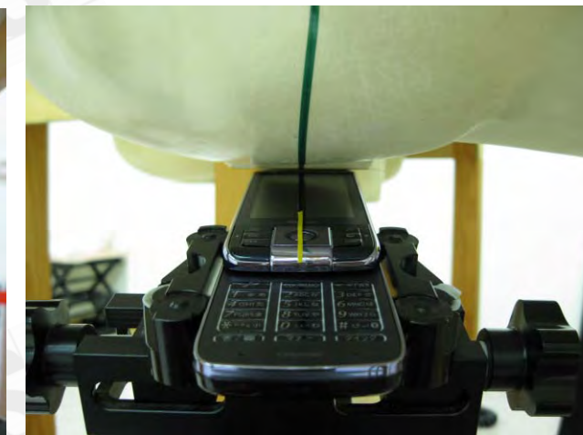
Fig.8 Right Head Section / Ear-Tilt Position(15°)_ Slider on
