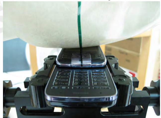
Fig.9 Left Head Section / Cheek-Touch Position_ Slider on
