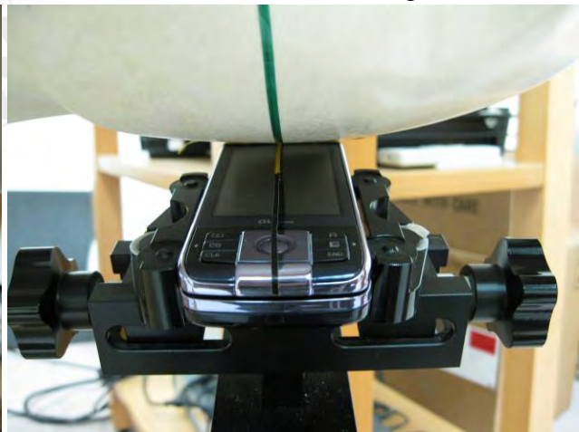
Fig.6 Left Head Section / Ear-Tilt Position(15°)_ Slider off
