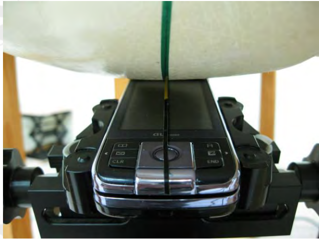
Fig.4 Right Head Section / Ear-Tilt Position(15°)_ Slider off
