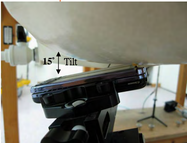
Fig.6 Left Head Section / Ear-Tilt Position(15°)_ Slider off
