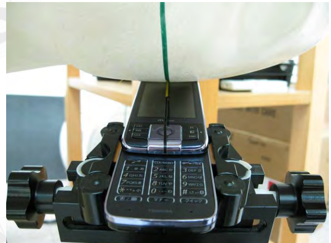
Fig.10 Left Head Section / Ear-Tilt Position(15°)_ Slider on
