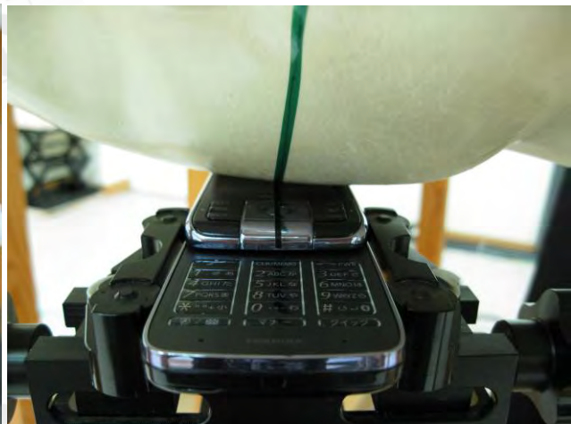
Fig.7 Right Head Section / Cheek-Touch Position_ Slider on
