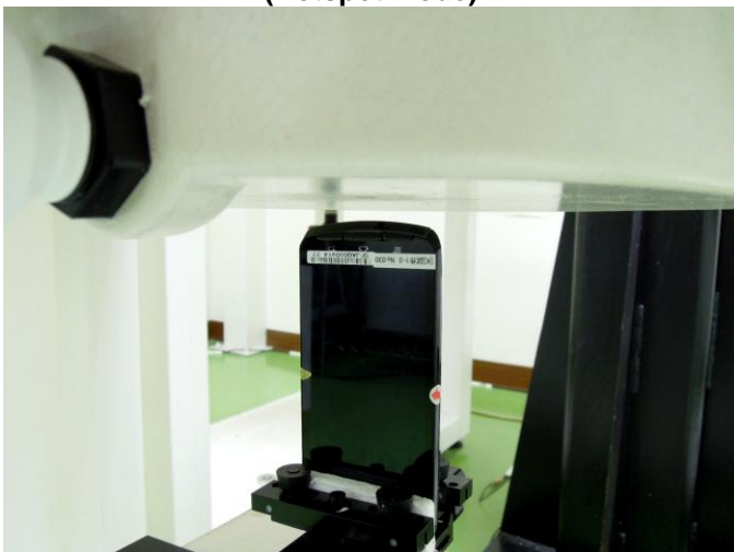
Bottom Side of EUT with 1.0 cm Gap (Hotspot Mode)
