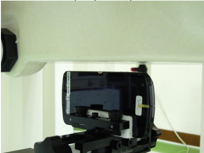
Left Side of EUT with 1.0 cm Gap (Hotspot Mode)
