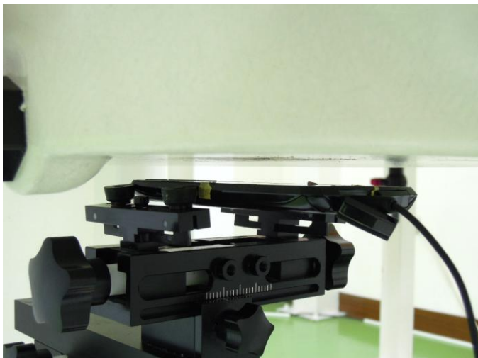
Front Face of EUT with 1.0 cm Gap (Body Worn Mode)
