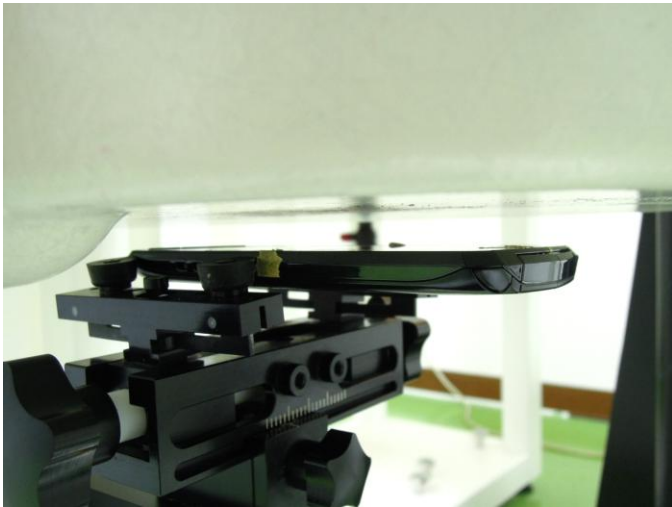
Front Face of EUT with 1.0 cm Gap (Hotspot Mode)
