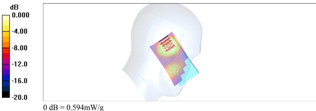
**#08 GSM1900\_Left Tilted\_Ch512\_2D****DUT: 190327**
