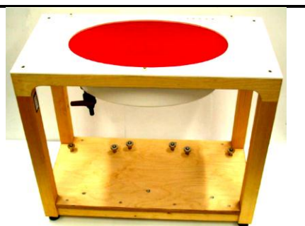
Fig 5.10 Photo of ELI4 Phantom
