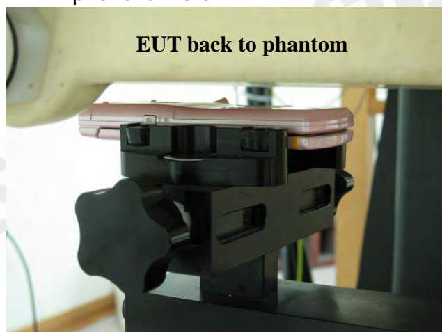
Fig.9 Body worn- EUT back to flat phantom and distance between flat phantom and mobile phone is 1.5 cm_ repeated with headset.
