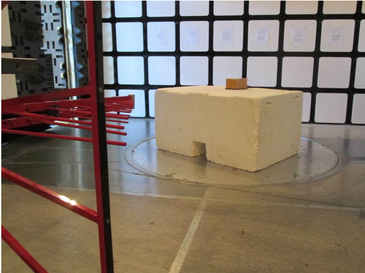
Test setup photo 2 Radiated measurements, 30 MHz – 1 GHz
