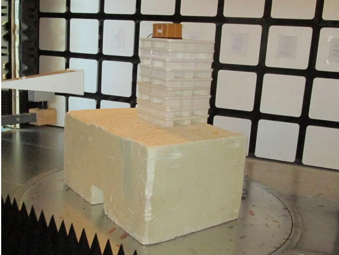
Test setup photo 5 Radiated measurements, 10 GHz – 18 GHz
