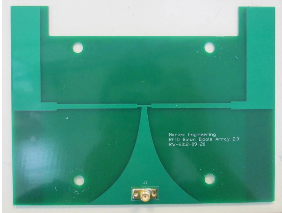
EUT – Internal view 14 900 MHz antenna, view 1
