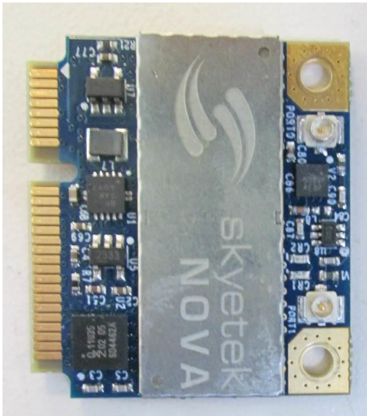
EUT – Internal view 7 900 MHz radio close-up, view 1
