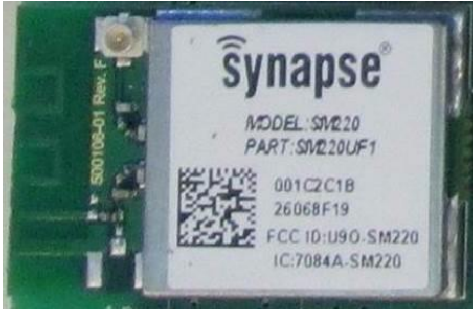
EUT – Internal view 10 2.4 GHz radio close-up, view 1
