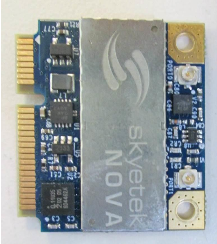
EUT – Internal view 7 900 MHz radio close-up, view 1
