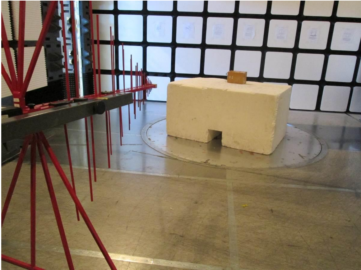
Test setup photo 2 Radiated measurements, 30 MHz – 1 GHz
