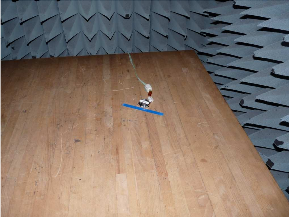
Photo 1: Test setup for radiated measurements (below 30 MHz)
