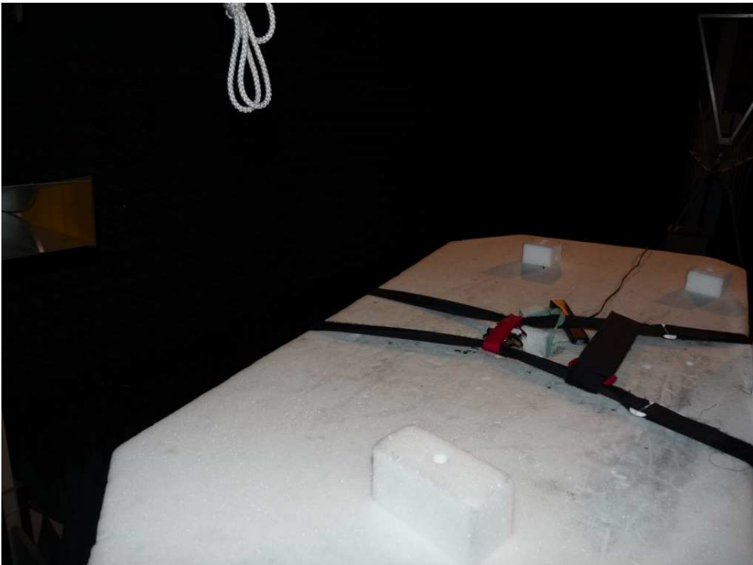
Photo 3: Test setup for radiated measurements (above 1 GHz)
