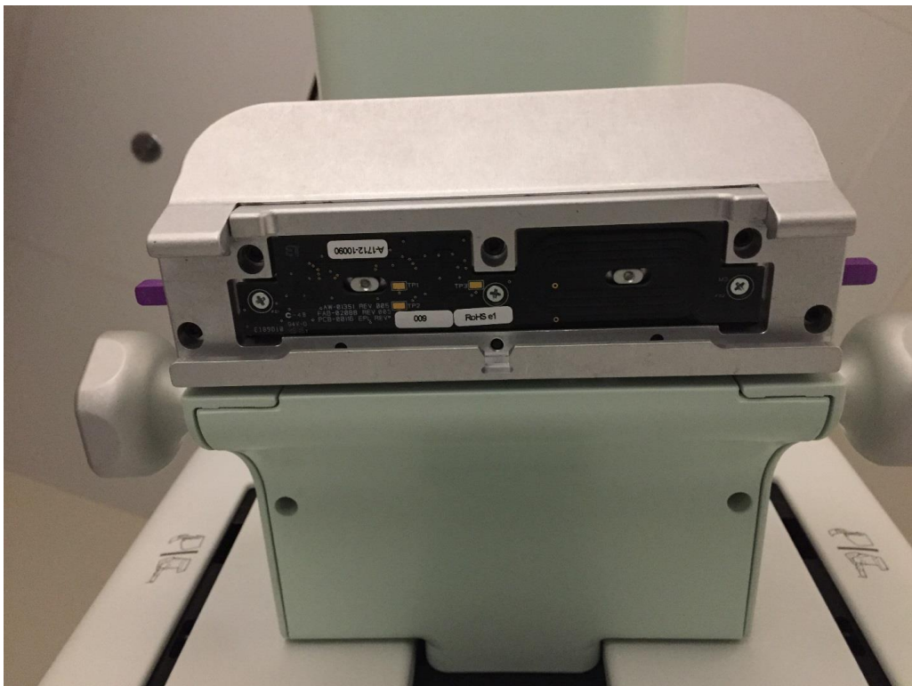
RFID Board shown installed in the Compression Device Assembly
