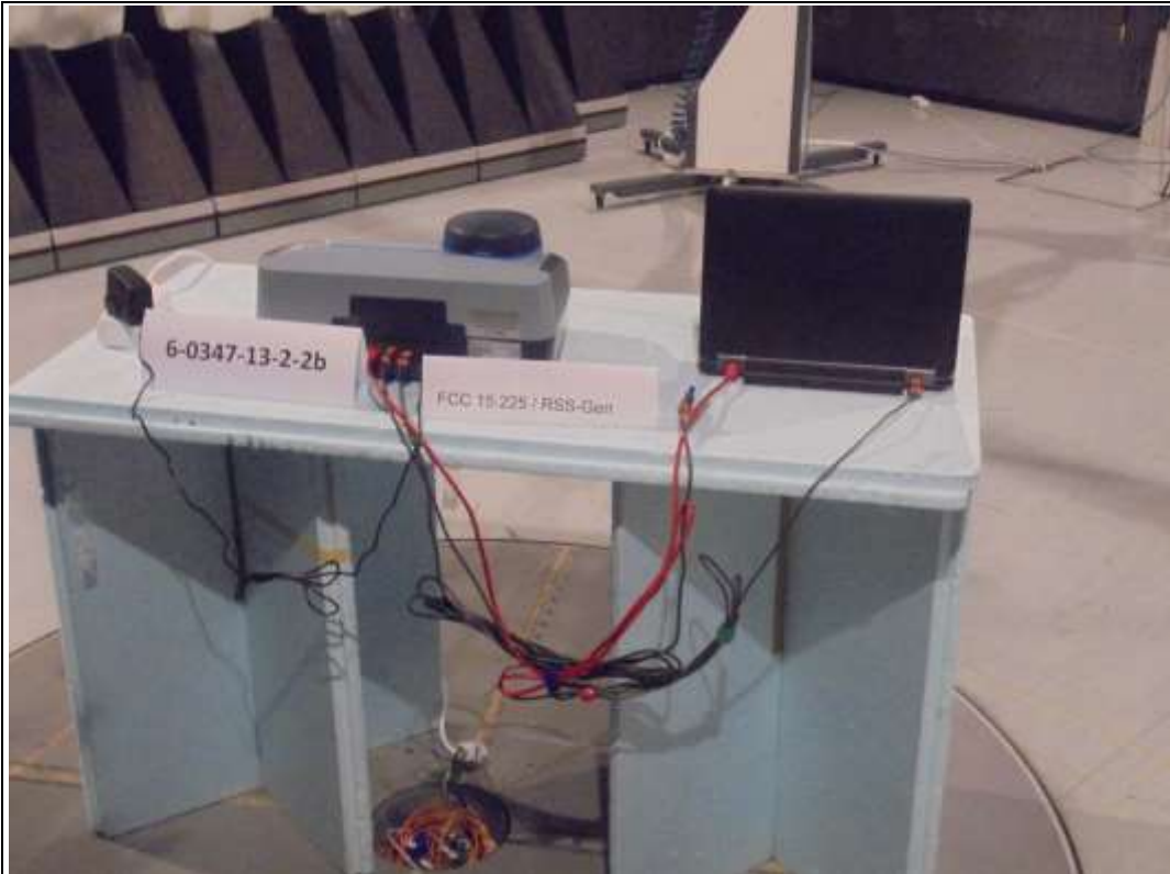
Photograph 3: Radiated measurements test set-up
