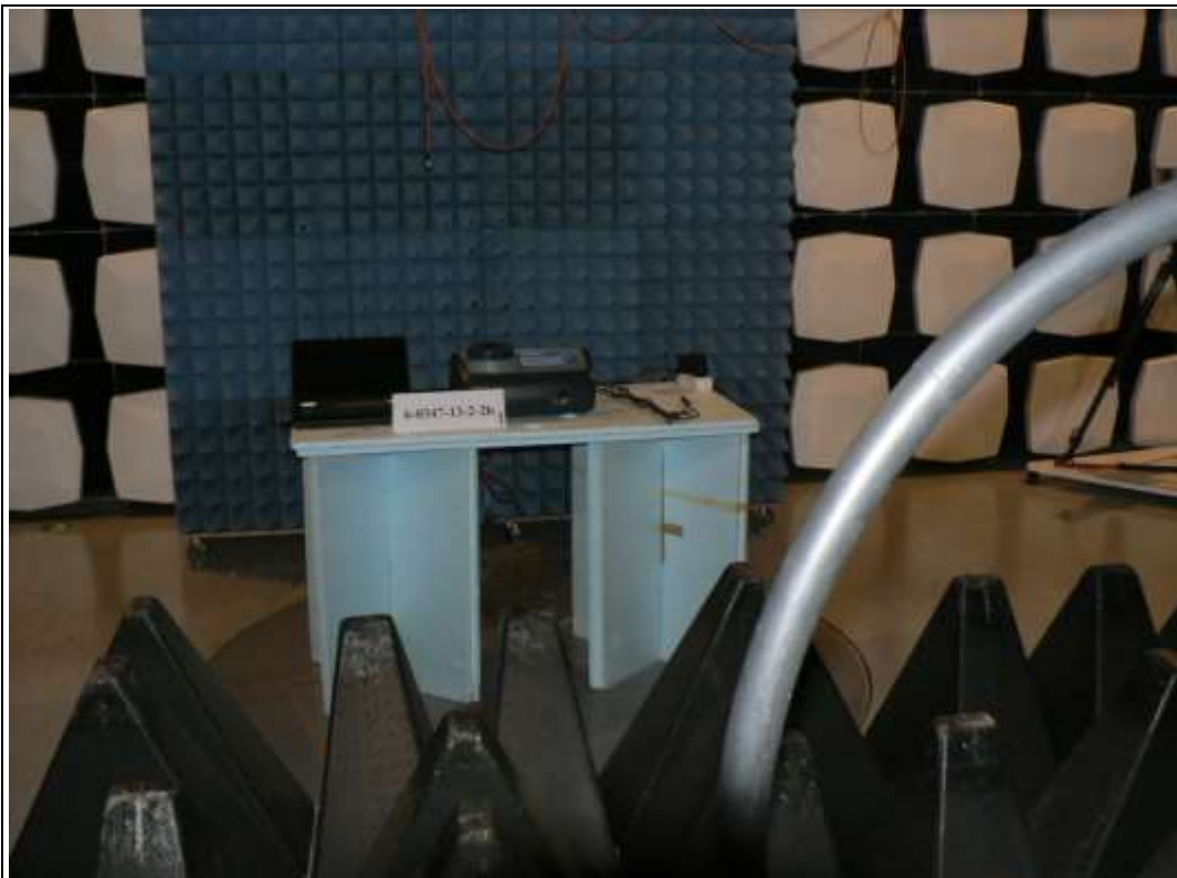
Photograph 4: Radiated measurements test set-up for magnetic fields
