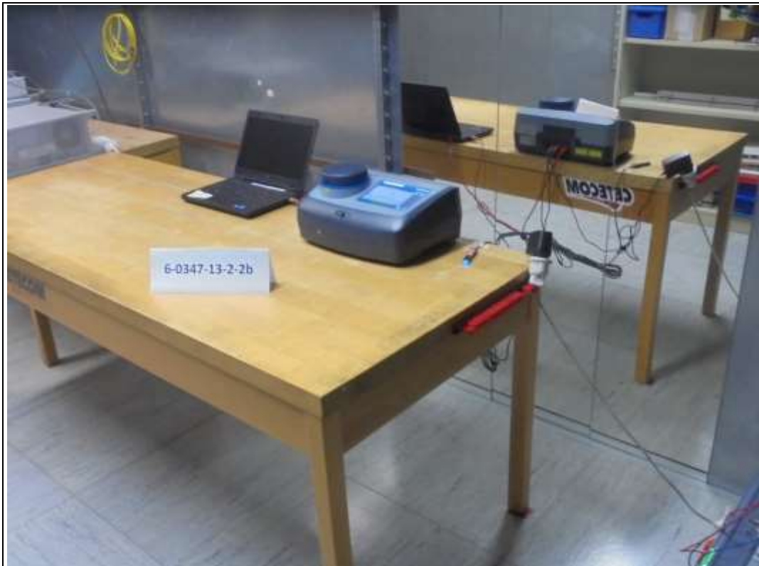
Photograph 1: Conducted measurements test set-up
