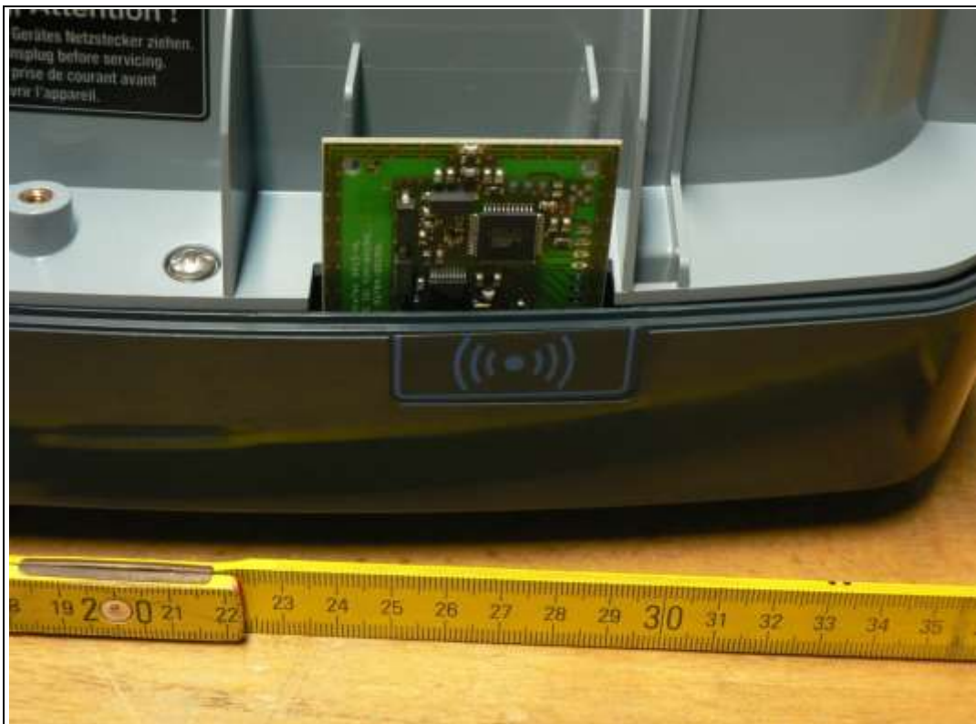
Photograph 4: Placement of RFID Module and Loop-Antenna inside device
