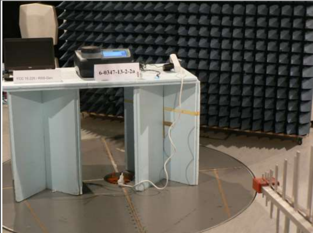
Photograph 3: Radiated measurements test set-up
