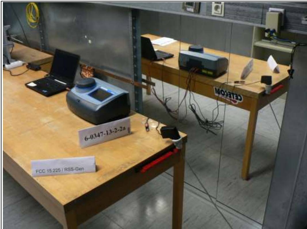
Photograph 1: Conducted measurements test set-up
