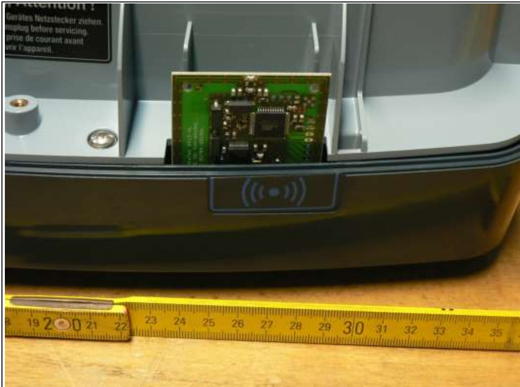
Photograph 3: Placement of RFID Module
