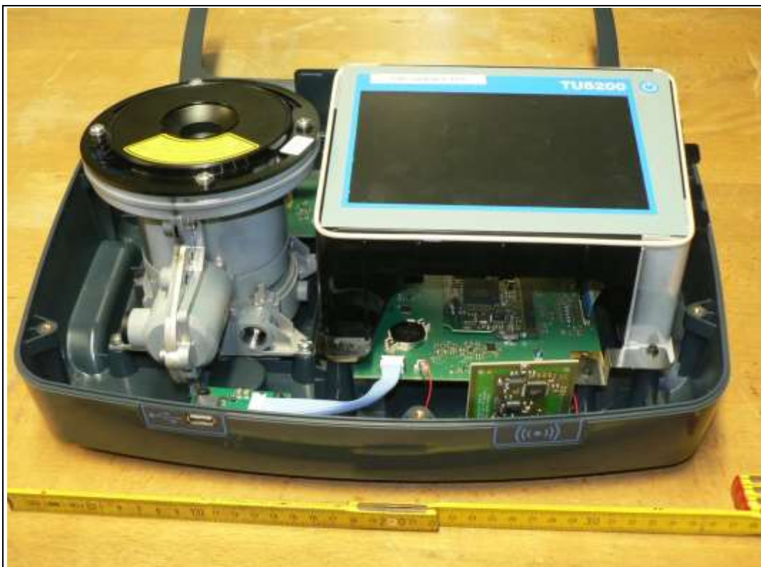
Photograph 2: EUT A - Cover removed
