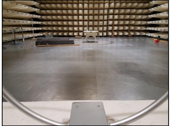
Loop-Antenna: EMCO 6502A (Correction factor @ 13.56MHz +9.5 dB)
