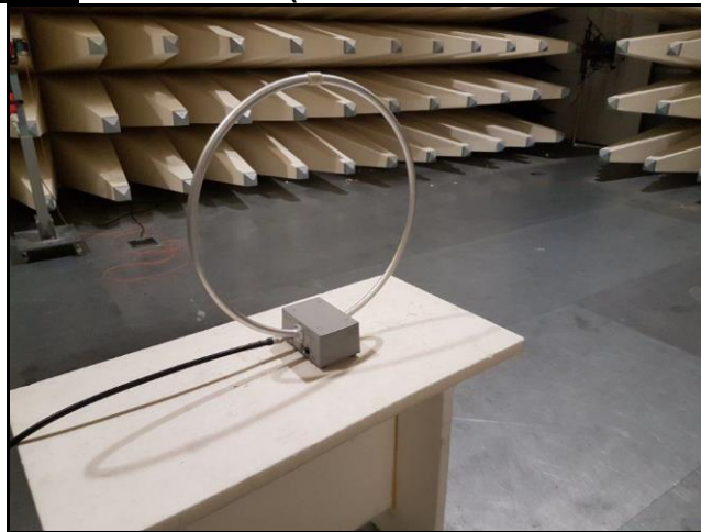
Loop-Antenna: EMCO 6502A (Correction factor @ 13.56MHz +9.5 dB)
