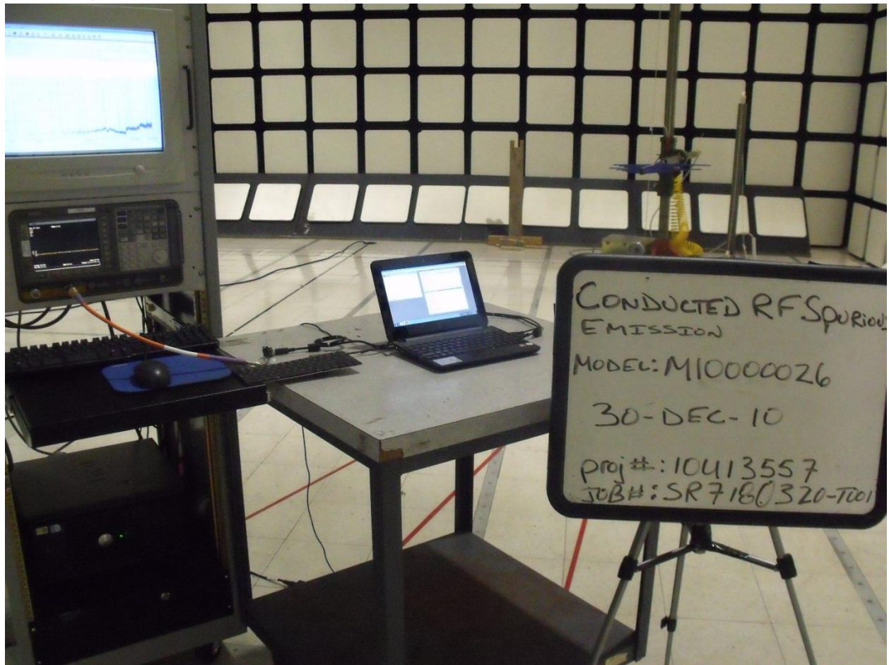
Test setup for Conducted – Antenna port
