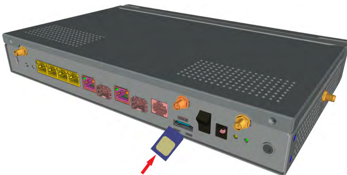
Fig. 35: Press to insert the SIM card into the tray
