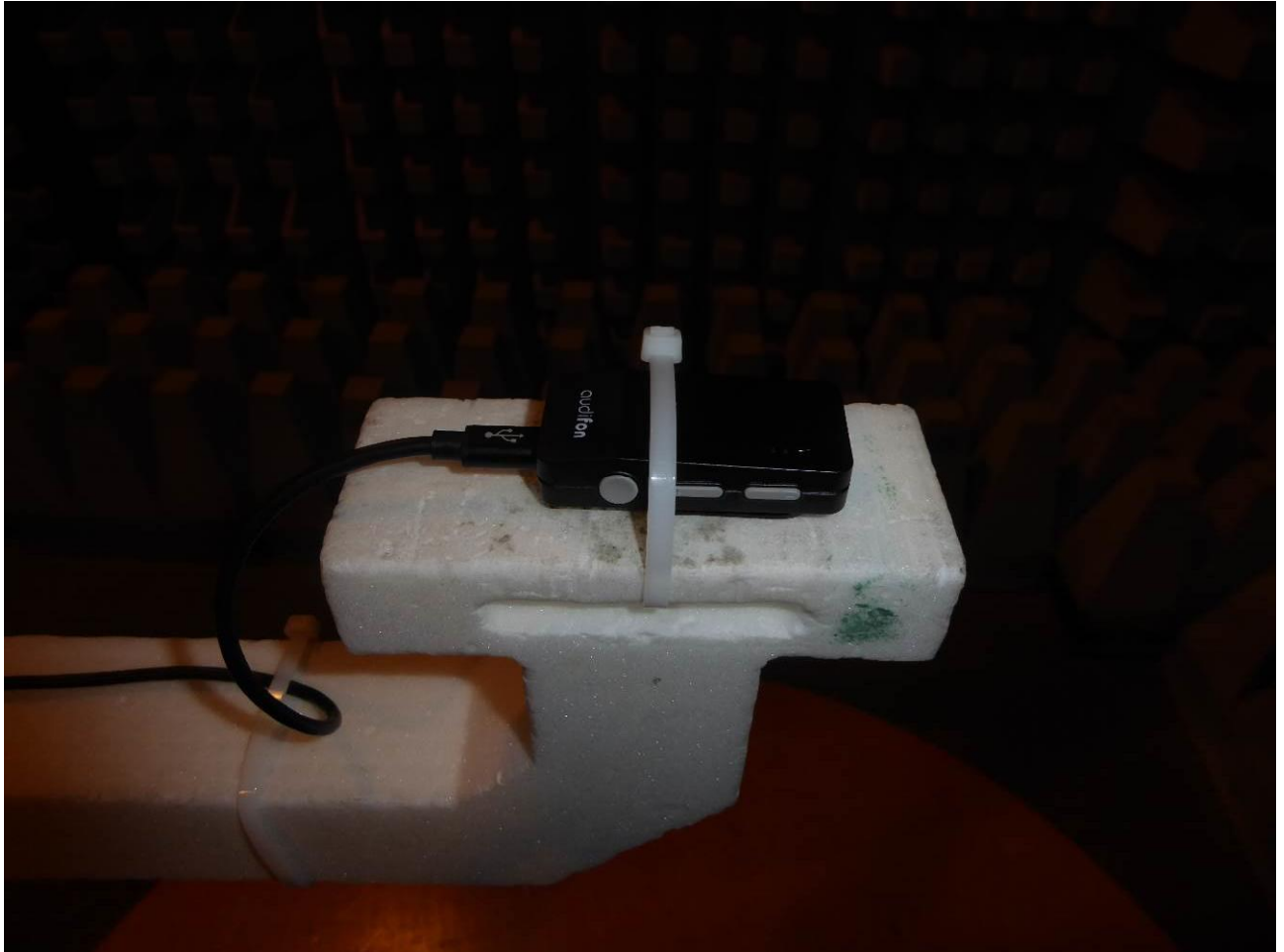
181631_247_BTLE_01.JPG: Test setup – radiated test in anechoic chamber
