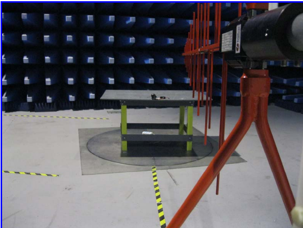
Radiated Emission Test Setup Rear View
