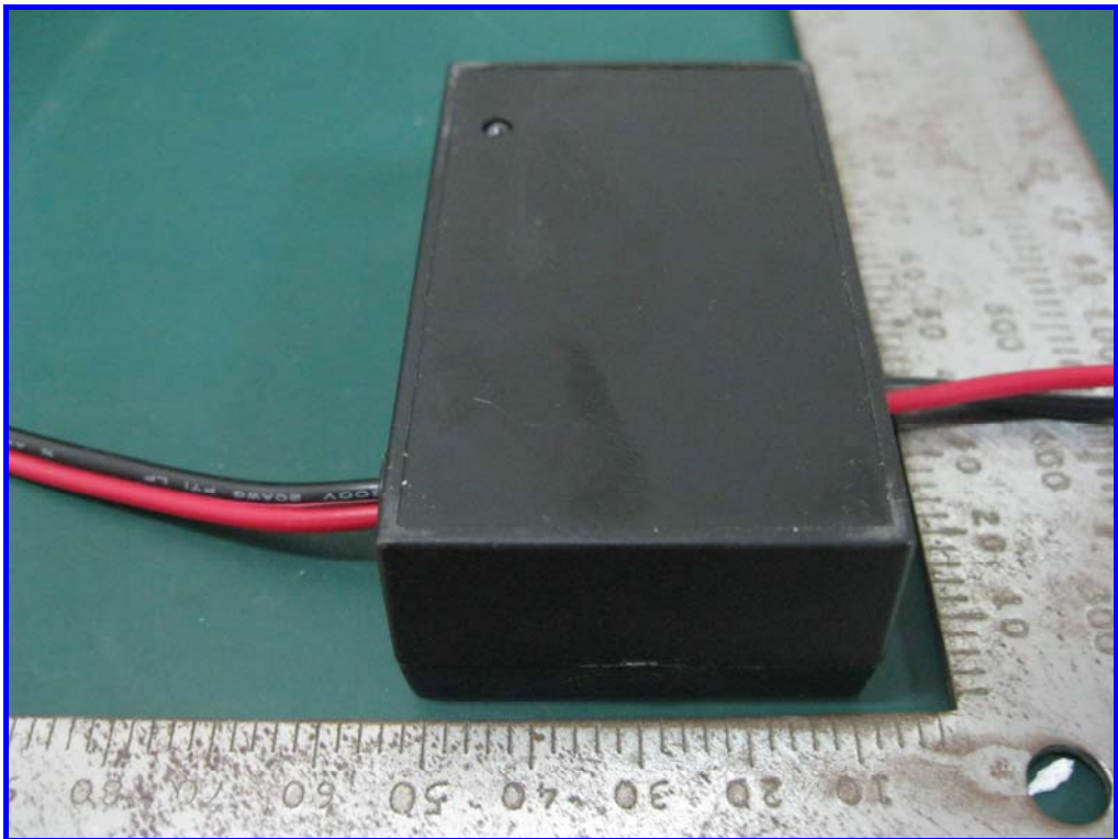
Bottom View of Universal Junction Box
